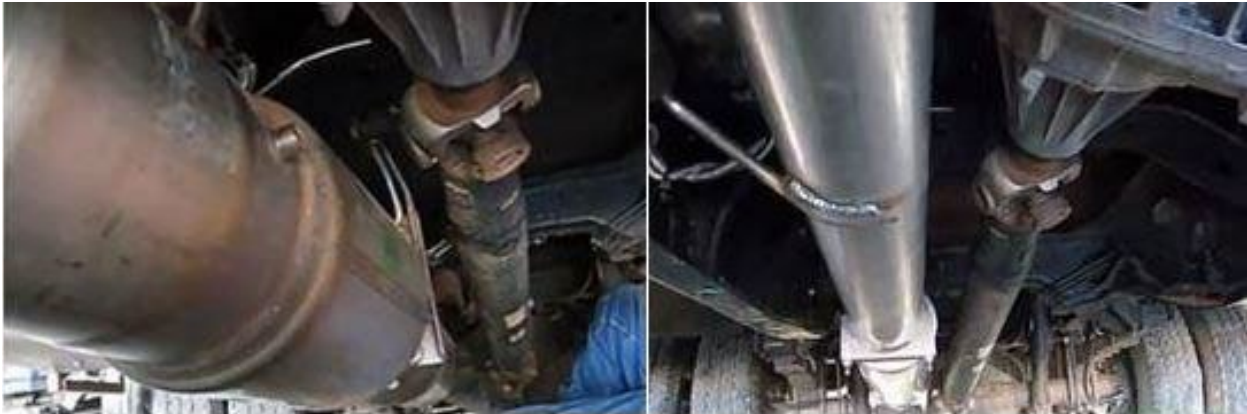
Figure 1: Example of tampering, which results in excess emissions
